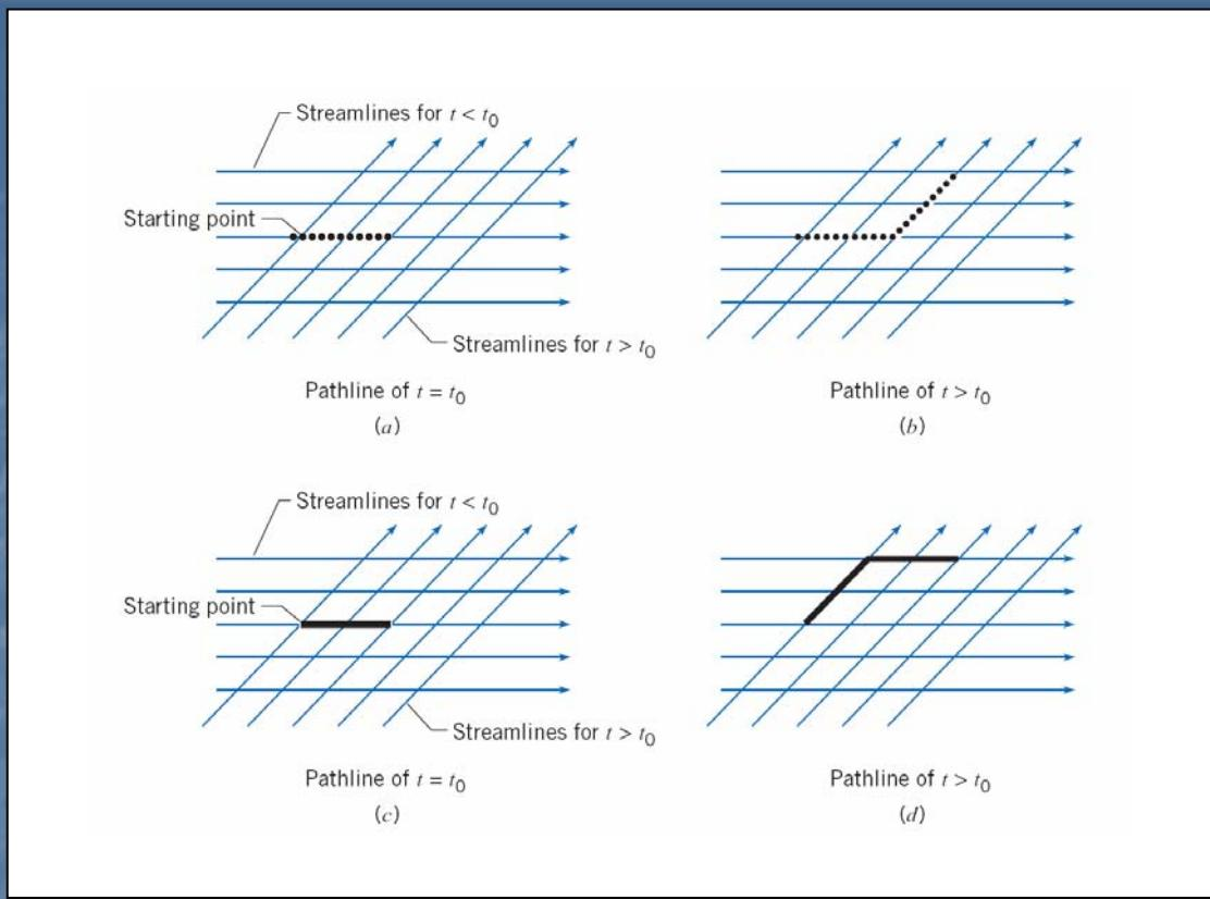
Streamlines: Is defined as the line or trace of a fluid particle in time within a flow as shown in Fig.12 .
